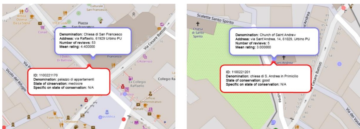
Figure 2: Examples of cases of mismatch (red dots refer to ICCD-mapped items, violet dots to Google Maps-retrieved ones): on the left, the potential error in pairing the objects is due to buildings' proximity in historic city centres, not allowing a match by coordinates; on the right, the impossibility of performing the match is due to the different denomination.
